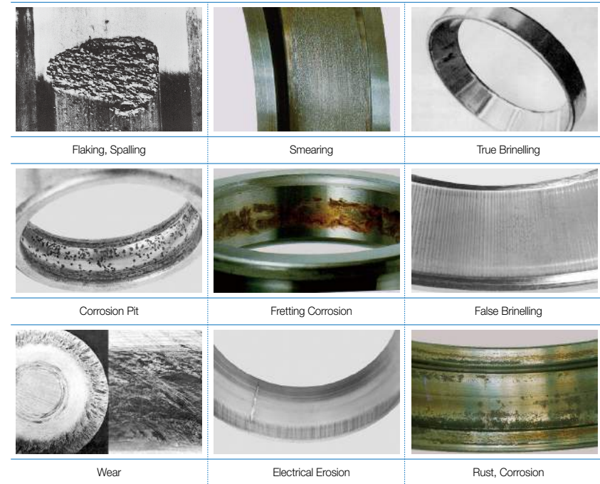
PIC 13.1 Bearing Damage
