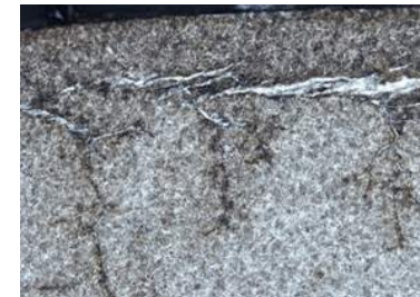
PIC 13.4 White Etching Area
