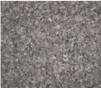
PIC 12.4 Induction Hardening Treatment (S55CR)
